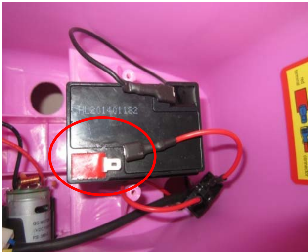
4. Open the seat, then connect the wire to the battery (red to red).
