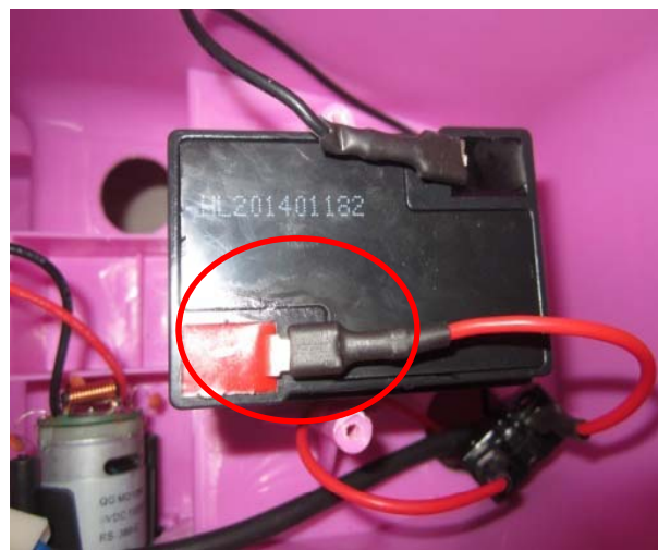
4. Open the seat, then connect the wire to the battery (red to red).
