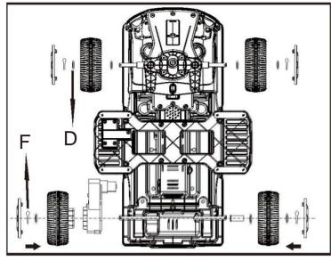
Turn over the car body,insert the rear axle into the car body,slide the motor on the rear axle,insert the rear wheel,make sure it matches up with the motor,set a shim,screw with a cotter pin,cover the wheel cap.
