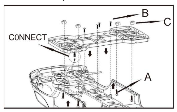
Turn over the car body, connect the lines of the pedal and the car, press the foot pedal on the car body, and fix it with screws. (5X20 Screw \*4 & M5 Mut \*4 & 4X10 Self tapping screw \*4)
