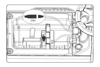
Remove the seat, connect the drive motor wire and power line, please note the polarity when connecting with battery wires, red to red, black to black. Finally, cover the seat and screw it.
