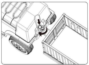
Hook the hook to the aft structure and turn the switch clockwise so that the container is attached to the aft.
