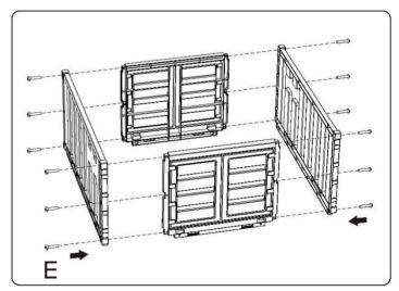
Assemble the 4 container panels together according to the picture and fix them with screws (4X8 Self tapping screw \*12)
