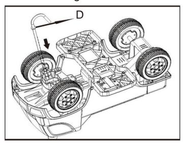
Put the steering lever with a shim to through the car's body..(10x18x1 Shim \*1)
