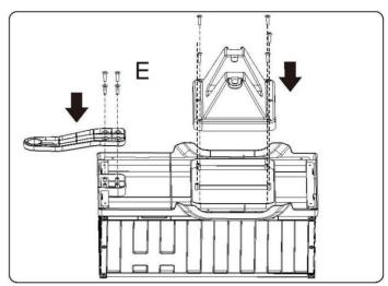
Install the shaft frame and coupling on the chassis and fix it with screws (4X8 Self tapping screw \*10 )
