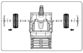
Insert the rear axle into the axle frame, insert the sleeve, gasket and normal wheel in the installation sequence, install the gasket again, tighten with the split pin, and close the wheel cover.
