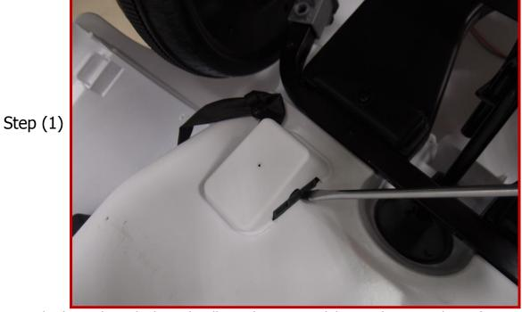
Upside down the vehicle and pull out the Foot Pedal cover by screwdriver from right side
