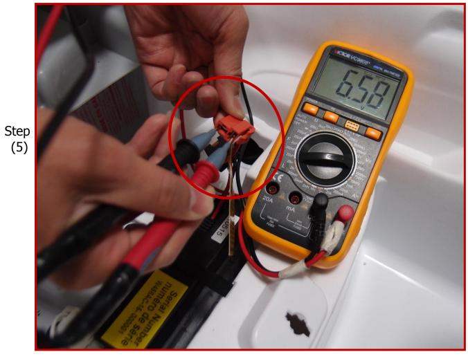
Reading Judgment:  $6.0 \text{ V} \sim 6.5 \text{ V} - \text{Good condition}$
