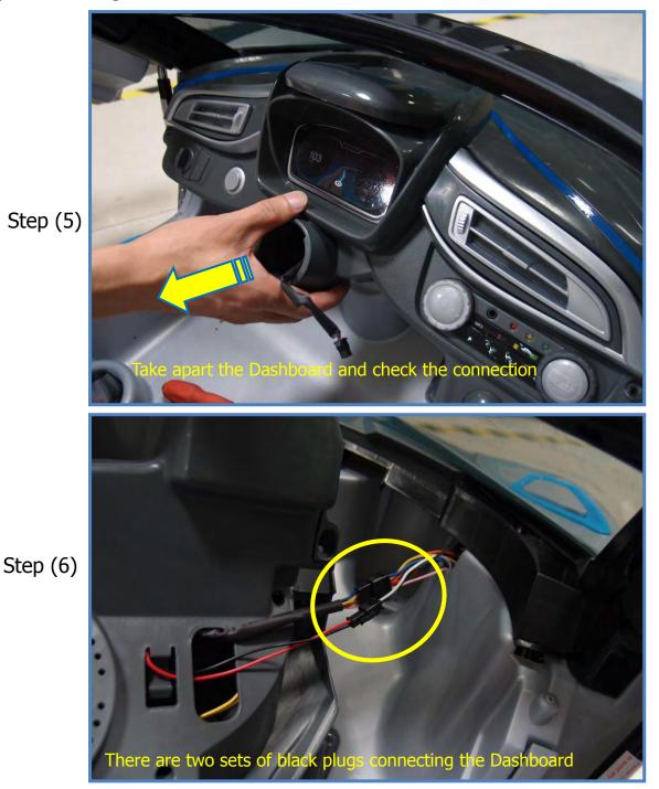
If the problem is address and fixed, reverse above steps to re-assemble the vehicle. Or unplug the connector and continuous as below steps when you need to further check the wiring inside Dashboard.
