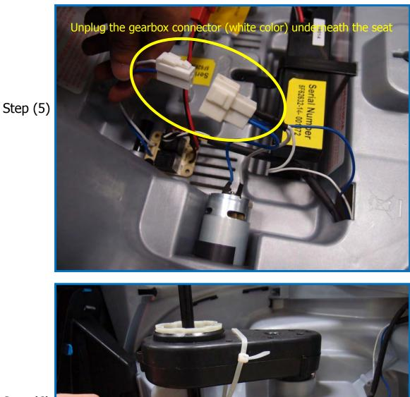
Cut the cable tie to release and remove the gearbox
