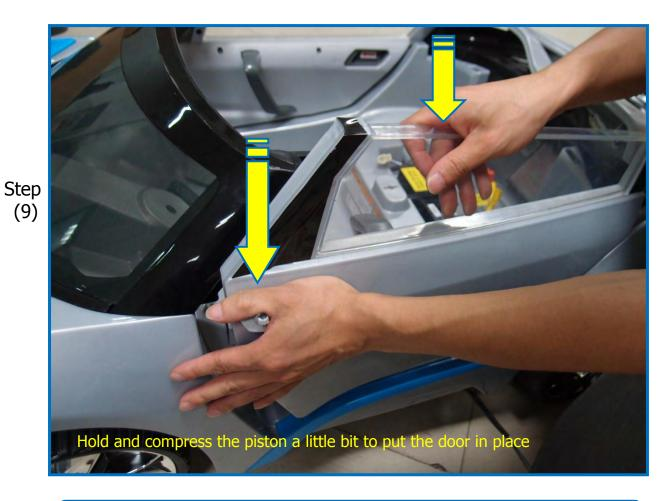
Reverse the screwing procedures to re-assemble back the vehicle
