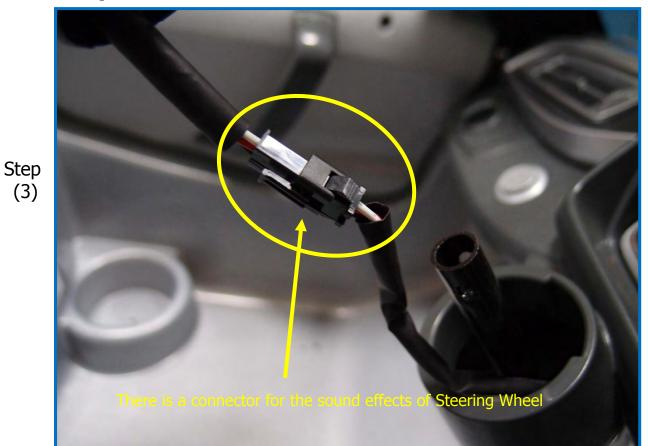
Unplug the connector and continuous below steps if you need to check the wiring inside Dashboard. Otherwise, reverse above procedures to re-assemble back the vehicle
