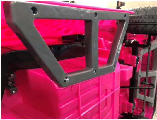
Step 1 (Turn over the car and take down the gray and black plastic parts as shown)
