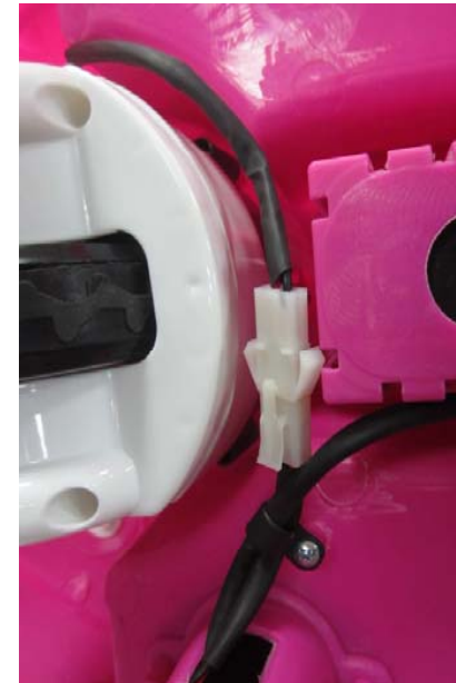
7. Turn the vehicle body, then check the plug if is it connected.
