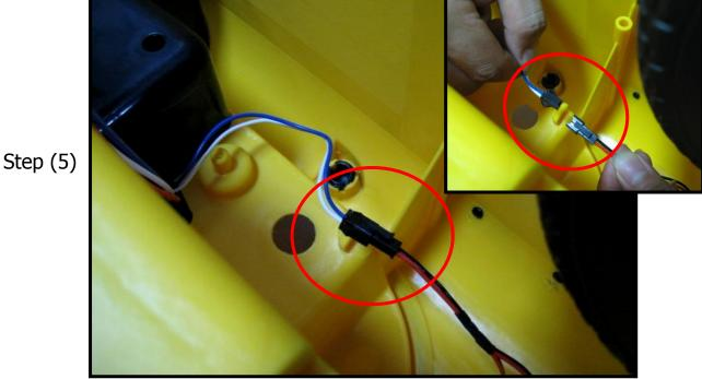
Unplug the Headlights connector plugs located at middle of bottom side
