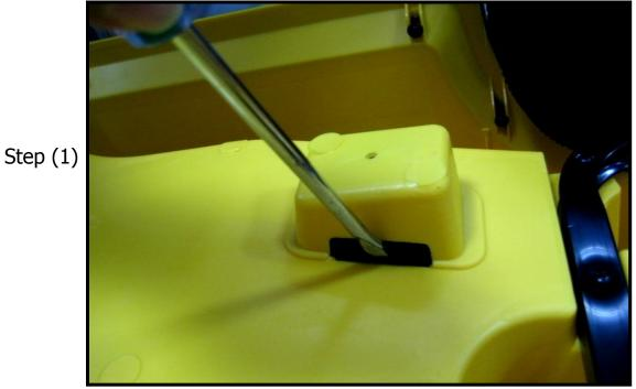
Turn over the vehicle and pull out the Foot Pedal cover by screwdriver from right side
