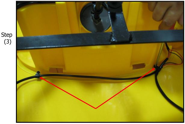
Unscrews two wiring clips to remove the Headlights Assembly
