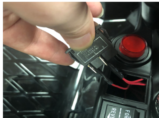
Step 2. Check the light on-off switch
