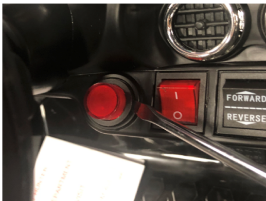
Step 3. Check the power switch
