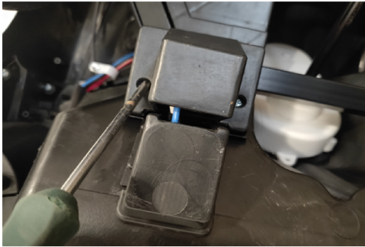
Step 1. Check the connection of pedal switch
