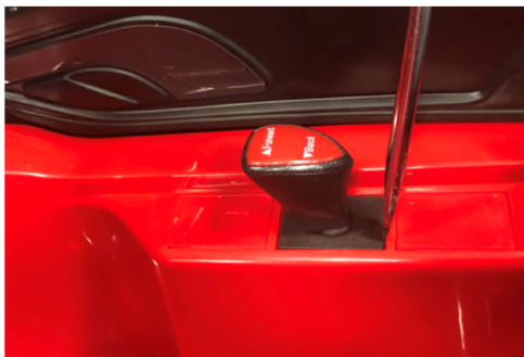
Step 2. Check the connection forward & reverse switch
