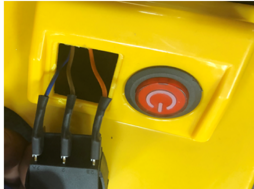
Step 1. Check the forward & reverse switch
