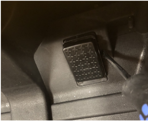
Step 1. Check the connection of pedal switch
