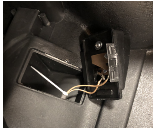
Step 1. Check the connection of pedal switch
