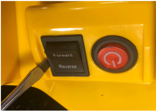
Step 1. Check the forward & reverse switch
