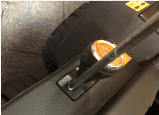
Step 2. Check the connection of rear bucket switch
