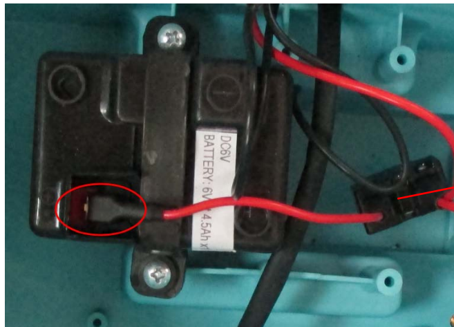
5. Connect the red wire of battery to the positive terminal.
