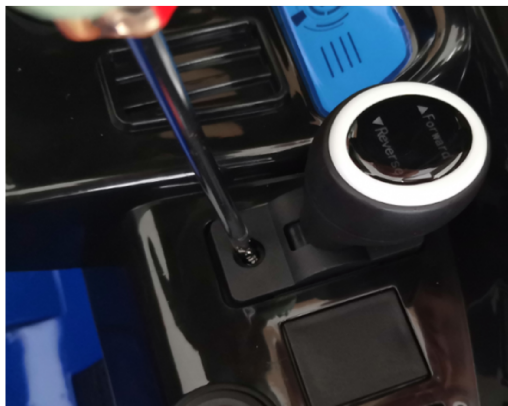
Step 2. Check the connection forward & reverse switch
