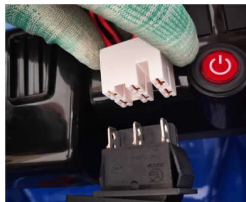
Step 2. Check the connection forward & reverse switch
