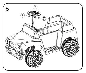
5. First, screw down \*7 screw from the the steering wheel and then aim the hold on the steering wheel to the steering rod, the steering wheel of the hole in the direction of the hole on the rod, and then fixed with \*7 screw.
