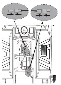
6.Plug the body's two core motor plugs each other, and then put the battery's red plug into the battery.
