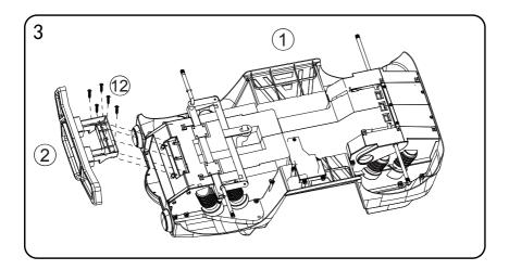
3. First put the front bumper in the direction shown in the corresponding position of the body, and then fix it with five screws.
