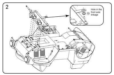
2.The Front Axle was factory assembled, but it need to be reset when you begun assembing. Turn the vehicle body over fit the front axle onto the front side of vehicle. If the side support does not seem to fit, change the other one and try again! Then tighten eight Ø4\*12MM round head screws to secure it with a screwdriver.
