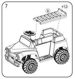
7.Insert the card in the front of the seat into the hole of the body and screw it up with one screw.
