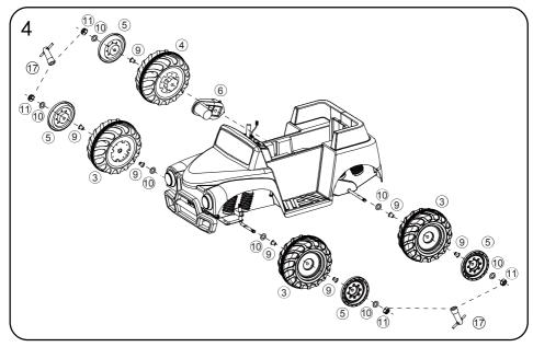
4.Each component is arranged in the front and rear shafts in sequence according to the instruction of the drawing, and then tighten the nut with a wrench
